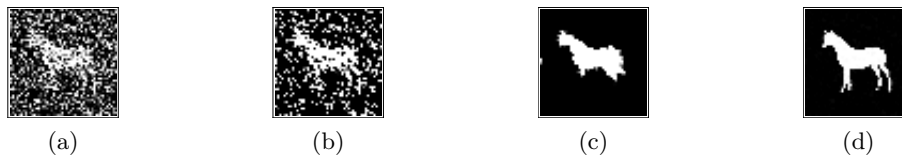
Fig. 7. Binary image segmentation of a horse: (a) noisy input, (b) only continuous cuts with high scale resolution \alpha = 0.1 , (c) only continuous cuts with low scale resolution \alpha = 0.3 , (d) coupled shape prior with high scale resolution \alpha = 0.1 . Without prior a high resolution (b) can not filter out noise, with low resolution (c) details (legs) are lost. The prior can help to distinguish noise and details.
